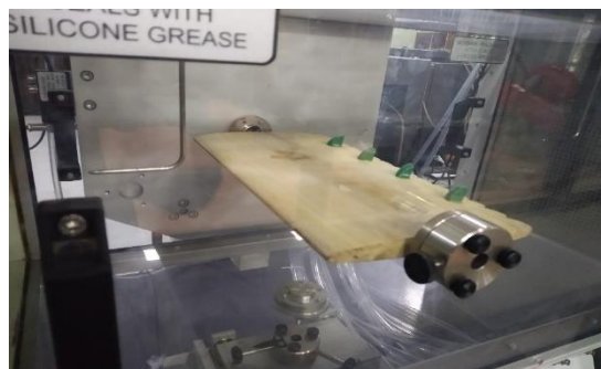
Fig. 08: Working section of the wind tunnel
