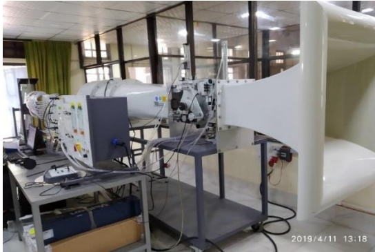
Fig. 07: AF100 subsonic wind tunnel in CUET lab
