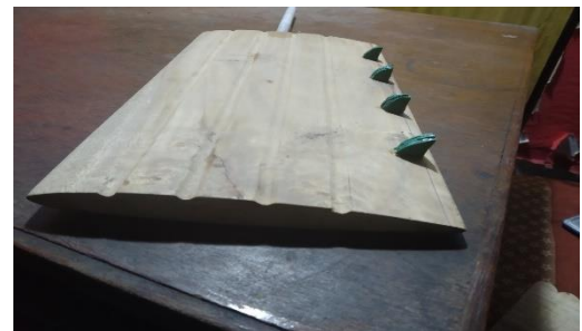
Fig. 06: Fabricated NACA0010 airfoil wings with surface modifications and vortex generators
